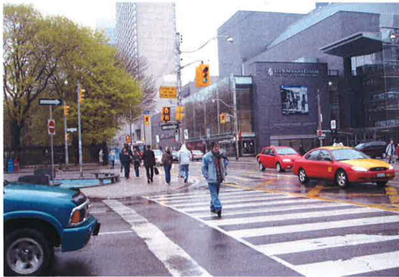
Example of an At-Grade Roadway Crossing Utilizing “Zebra Stripping”
