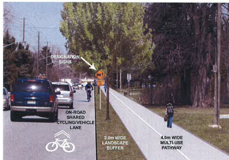
Example of a How the Preferred Design is Likely to Look in the Southern Part of the Study Area. Note: The Multi-Use Pathway, Landscaped Boulevard and Shared Outside Lane
