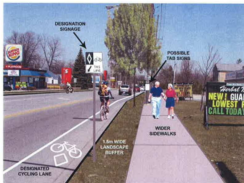
Example of How the Preferred Design is Likely to Look in LaSalle’s Town Centre Area. Note: The Sidewalk, Landscaped Boulevard, and Designated Cycling Lane.
