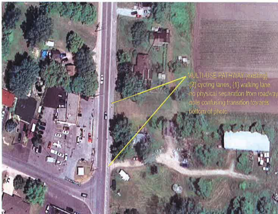
Aerial view of Malden Road at Reaume Road (see notes on image above.) (Photo taken from Google Earth.)
